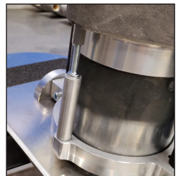
Ill. 2. Depth stop pin in use
